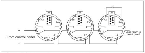
Schematic Wiring Diagram - XP95/Discovery mounting base
