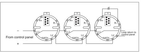
Schematic Wiring Diagram - XP95/Discovery mounting base
